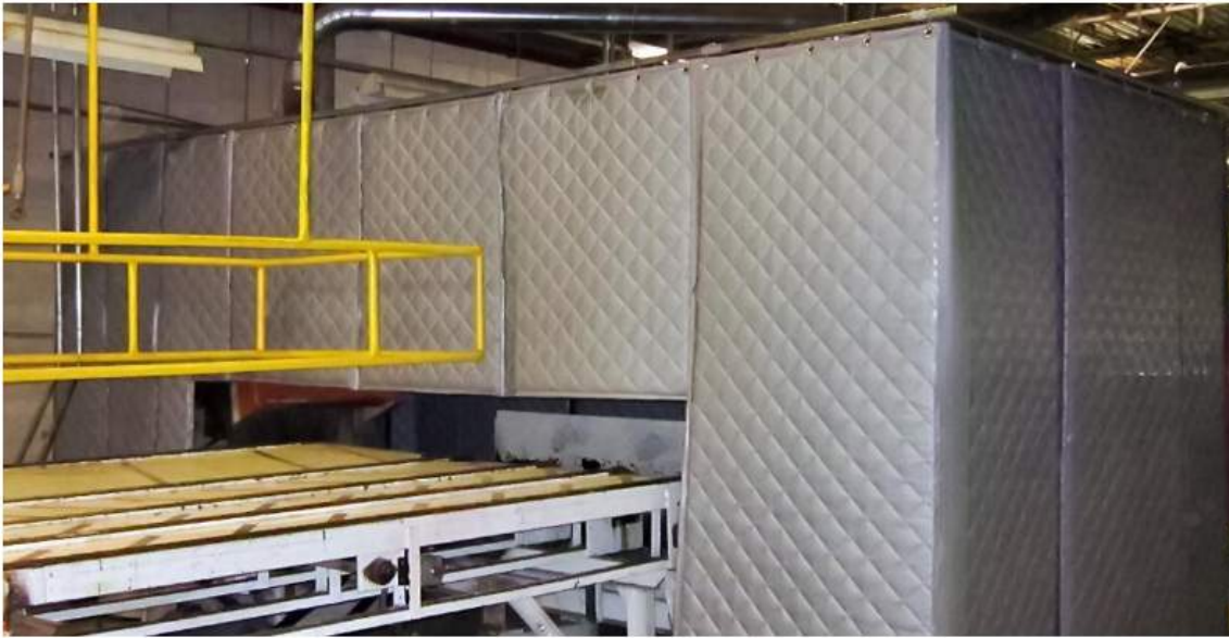
Modules are designed as independent units and can be soundproofed to block noise once they are assembled together.
