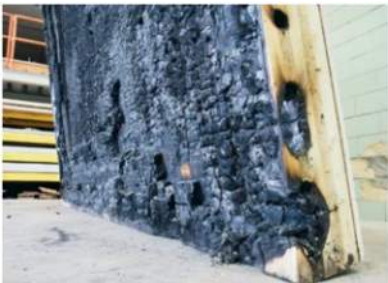
Figure 29: Wall assembly after testing showing the depth of charring on the exposed side. NRC (2014) Fire Endurance of Cross-Laminated Timber Floor and Wall Assemblies for Tall Wood Buildings.
